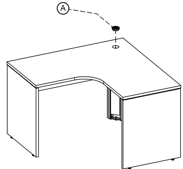
PARA FINALIZAR APÓS MONTAGEM COMPLETA DA MESA INSERIR O PASSA FIO (A).
